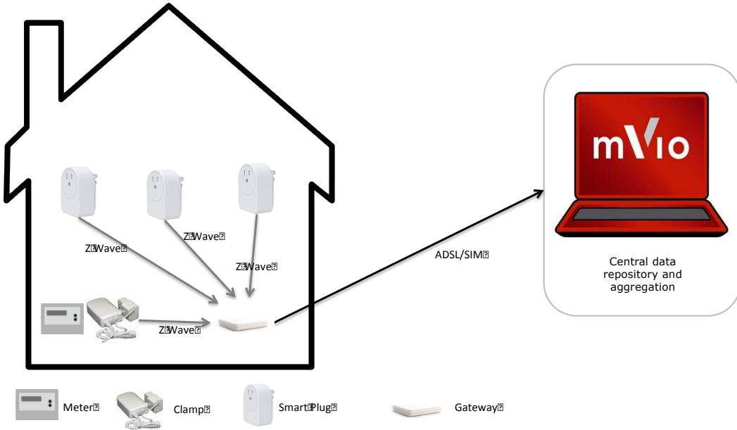
Diagram 1 – Typical installation (with smart plugs), showing data flow back to mVio via the gateway using Z-Wave and ADSL/SIM.
